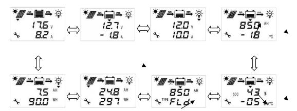
The following data can be adjusted: battery capacity AH, battery temperature compensation, battery type. On read status, press K1/SET for setting data.
