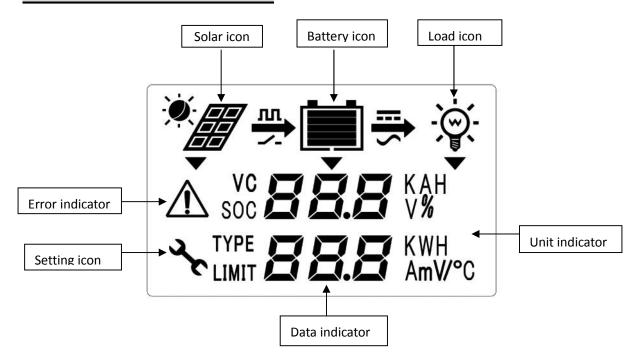
• The two LED indicators above the LCD show that battery is charging, and a red indicates error conditions. The LCD has three different brightness levels. After any button is pressed the display will be in high brightness and backlight. After 15 seconds the display will switch to a lower brightness, and after an additional 15 the backlight turns off.
